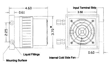
\* Dimension does not include hardware, Insulation. Dimensions are in inches.
